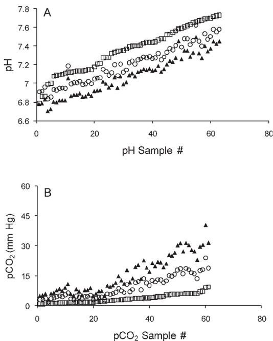
FIGURE 2.—Values for (A) pH and (B) ( $p\text{CO}_2$ ) in full distribution (using pooled data from both sandbar sharks and smooth dogfish) in ascending order for the radiometer blood gas analyzer at 25°C (open squares); i-STAT PCA values manually converted to 25°C using equations from Mandelman and Skomal (2009; open circles); and raw i-STAT PCA values at 37°C (triangles).
